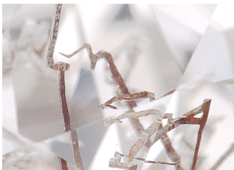
Incredible dissolved dislocations in a natural type IIa diamond. Photo LFG
